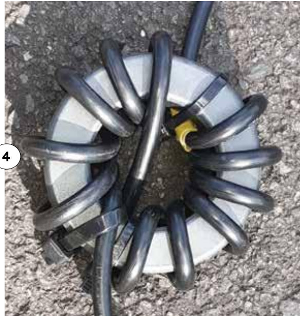
You can make an effective RF choke for an antenna system by wrapping coaxial cable through a sizable core.
