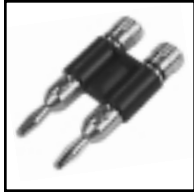
30-604-RD 30-604-BK Dual gold banana plugs. For up to 8 gauge wire. Black or red. .15" cable opening. 0.75" centers.
