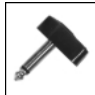
30-407 1/4" mono right angle plug, black bakelite. Solder terminals w/cable clamp. .28" cable opening.
