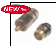
NEW Item 30-354 RG59 30-354 RG6 75ohm gold RCA connector. Recessed barrel provides a low profile when inserted into a female jack. Solder center pin at base of connector, fold shield over PVC, a 2 piece twist type compression fitting is used to secure the shield to the connector.
