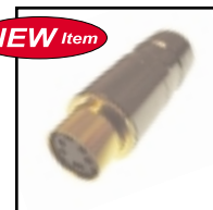
30-618 SVHS inline female jack. Solder type connector. Accepts 5-7mm cable. Black chrome body with gold plated connector.
