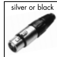
30-528-SL 30-528-BK XLR 3-pin female plug, twist-on strain relief. .15" to .3" cable opening. No tools required for assembly or disassembly. 4 piece construction. Internal compression style cable strain relief.
