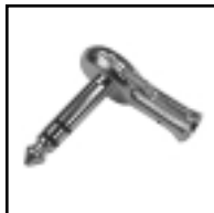
30-408A Flat right-angle, shielded 1/4" 3- circuit stereo phone plug in metal case. Solder terminals. .29" cable opening.
