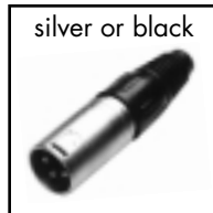
30-529-SL 30-529-BK XLR 3-pin male plug, twist-on strain relief. .15" to .3" cable opening. No tools required for assembly or disassembly. 4 piece construction. Internal compression style cable strain relief.
