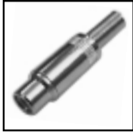
30-429 Shielded, nickel plated RCA-type inline jack w/cable clamp. 3/8" dia., 1" long. .21" cable opening.
