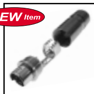
30-505-6 Pro quality SVHS 6-pin connect for up to 5.7mm cable. Metal housing with gold pins and gold strain relief. .27" cable opening.
