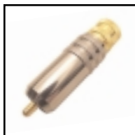
30-607-BK 30-607-RD Locking RCA plug for up to 8 mm wire. With black or red band. Teflon insulator. .35" cable opening.
