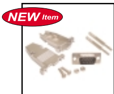
30-556 Solder type HD- 15, 15 pin male with metal hood and hardware. Accepts cable up to 11mm, .433".
