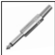
30-536 1/4" Mono phone plug w/screw terminals and strain relief spring. .25" cable opening.
