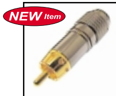
NEW Item 30-302 Gold plated RCA plug with teflon insulator for 6-8mm cable. Specify black, red, white or yellow band. Gold plated. .35" cable opening.
