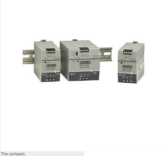
lightweight DIN Rail power supplies come in output voltages from 5 to 48 Vdc and power ratings of up to 100 Watts. T hese extra small, efficient units are designed specifically for the industrial environment. Ea ch unit is rated from -10°C to 70°C, with no derating necessary until above 60°C. Many extra "industrial" features are standard for the SDP PowerBoost™ overload circuitry can start up industrial loads (i.e. motors, relays, solenoids and DC-DC converters), that can cause ordinary power su
