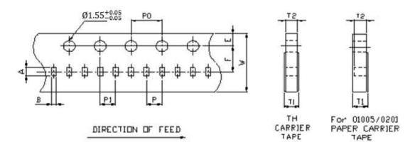
Remark: Pitch tolerance over any 10 pitches of Po is  $\pm$  0.2 mm
