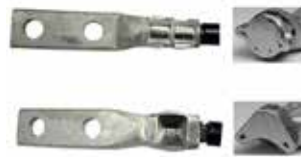
Circumferential compression is solid and symmetrical. No sharp flash.
