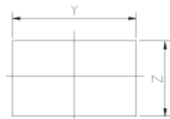
Snap-in Panel Cutout X=Panel Thickness
