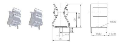
Description: PCB Clips for fuse, including EV325-3EC (1 fuse with 2 clips).
