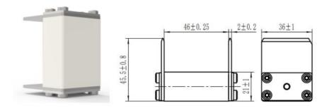
**Features:** Compact size, designed for ESS MSD. The typical rated voltage of fuses in MSD include DC250V, DC750V and DC1,500V with rated current range 21A~400A.
