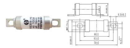
**Description:** Rated voltage DC750V/AC800V, rated current 10A-100A optional; Featuring strong current limiting and high breaking capacity [DC50kA (time constant 10ms)/AC100kA, power factor 0.2]; Product complies with RoHS and has CE, UL, and TUV
