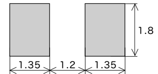
Land pattern for reflow soldering (reference dimensions)
