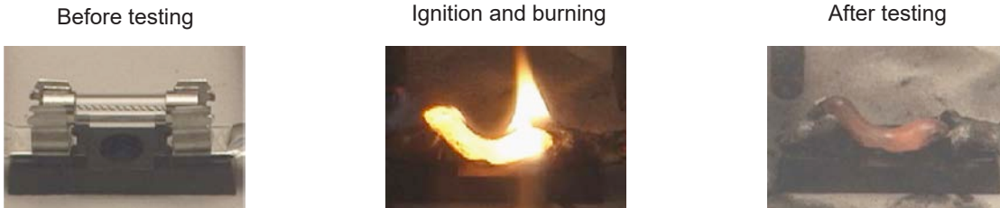
Example of a breaking test where the circuit voltage is higher than the rated voltage of the fuse
