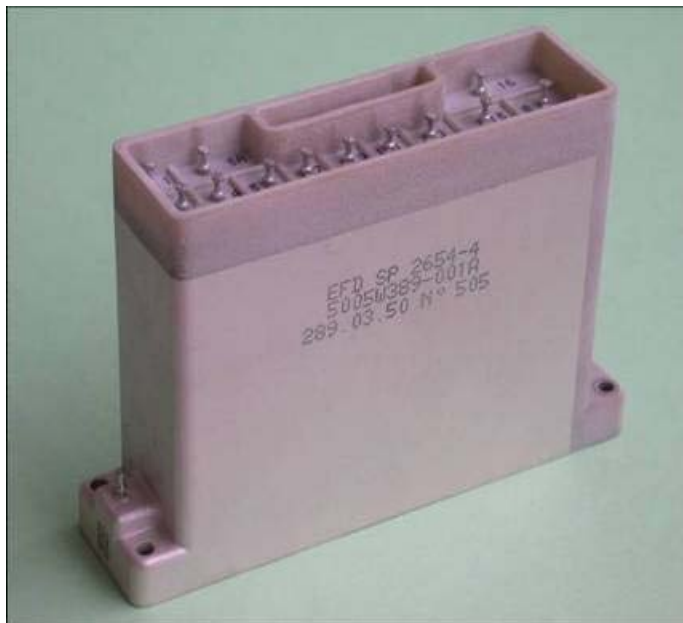
Space Application – On Board TWT Radar Custom design integrating 25 capacitors with 13kV total rated voltage Dimensions 102x25,5x70,5 mm Weight < 280 g
