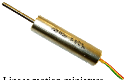
Linear motion miniature Plastic Film Potentiometer for AMOS 3 Plastic film, 0.1% linearity, Repeatability 10 µm
